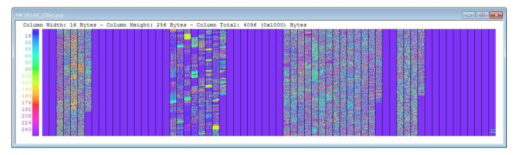
Now let's break down this image. Looking at the scale color scale on the left and applying that to the image, we can see that all the purple sections are just filler with a value of 255 (0xFF) and can be ignored. What we want to focus on are just the multicolored sections. In this example of a Ford Power Stroke calibration, you can see 4 distinct sections in the data.
