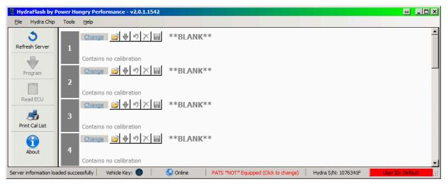
The lower-right corner of the status bar will display the current User ID and Serial Number of the Hydra<sup>™</sup> Chip. Unless otherwise specified, the User ID will always be the "Default" user. The Serial Number is used in situations where a custom files is built and encrypted to a specific chip.
