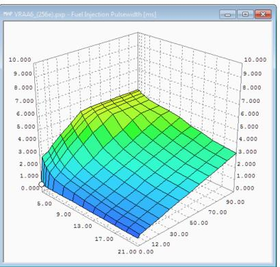
Some of the other options of the Map can be defined, such as the Z-Axis Angle (startup view angle, which is usually 45 degrees), the Units of the values, the Format (how many decimal places), and the Adjust and Alt Adjust values for using the +/- keys. These make editing the Map values much more intuitive, especially when in Graphics mode.
