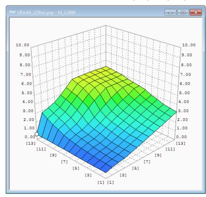
At this point, we still don't have any labels for the X-Axis or the Y-Axis. Those will need to be determined and properly linked to the correct Normalizers as well as having the Map properties set to allow Scaled Label Spacing for the Map to be correctly scaled visually.
