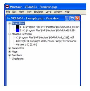
In this sample project, I've included a stock calibration as an overlay to use for comparison against the 60 HP Performance calibration. You should also notice that the Parameters, Maps, and Functions each now have a plus [+] symbol in front them. This indicates that there is modifiable data in each category.
