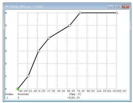
Even though the there is no explicit data point for "2" on the Y axis, this can be interpolated as a point halfway between 1 and 3 with values of -20 and 0. Since point 2 is halfway between 1 and 3, the assumed value for point 2 would be halfway between -20 and 0, or -10. This is how
